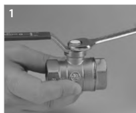
Remove the nut with the proper wrench
