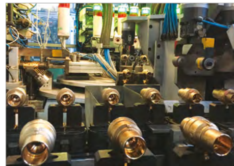
Automatic assembly with 100% in-line tests'
