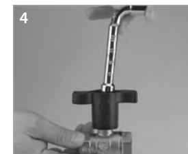
Tighten the nut completely using the proper socket wrench
